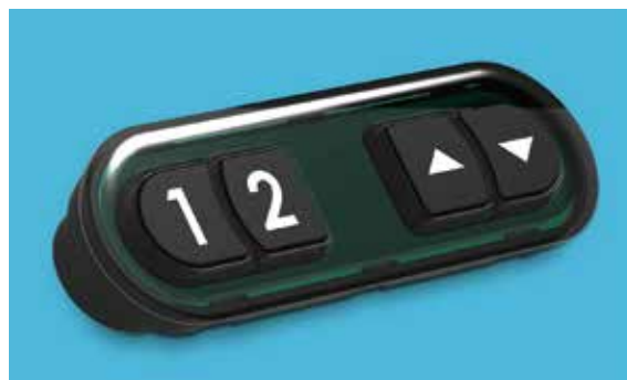
LM41C Control panel with up and down button and 2 individually assignable memory keys, to be mounted into a 6 mm deep milled recess
