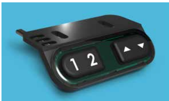
LM4LIP Control panel with up and down button and 2 individually assignable memory keys, for under-table mounting, water-jet proof, IP65
