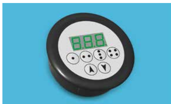
LD6R Control panel with up and down button and 4 individually assignable memory keys, digital height display, bore diameter 60 mm, to be mounted into a 6 mm deep milled recess
